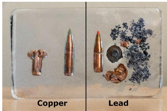
300 win mag solid copper (left) 300 win mag lead core with copper jacket (right). Photo by Mike McTee
